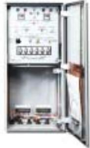
PST (Padmount Source Transfer) switchgear provides total transfer time of 6 cycles or less. PST uses the S control, and CI interrupters with quick-close / quick-open mechanisms. The S control is a time-proven device, which provides the timing and control logic required to perform the source transfer. Discrete SCADA contacts for remote operation, are provided as an accessory to the transfer S control.
