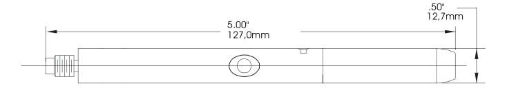
The **166LRF** loadbreak elbow probe is designed to be used with all the 15 kV class loadbreak elbow, such as 165/166LR, 167/168ELR, 167/168
