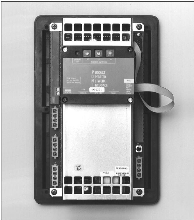
Figure 2-3 Communication Module - PONI (mounted)
